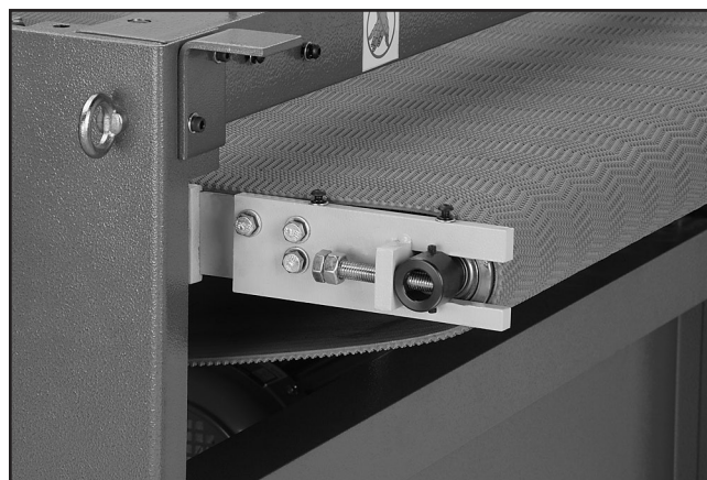
Figure 48. Conveyor belt loosened at the rear adjustment.
